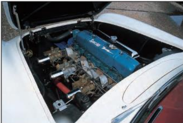
1953 Corvette 235.5-cid 150-hp inline six-cylinder engine
