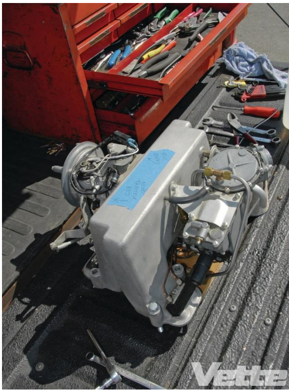
03 This particular '57 Corvette needed a quick swap-out of the fuel-injection unit in the pits, in time for race day
