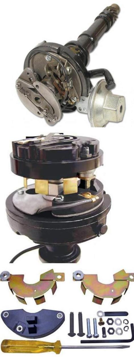
The **Lectric Limited** electronic ignition module kit replaces all the internal components; points, capacitor, clamp & screw and the lube wick, inside the Corvette distributor below. The original distributor, after installation, which was simple, still appears original. Other than needing a larger screwdriver to remove the distributor cap, tools needed were supplied with the kit. At disassembly, I found that points had started to burn after 19,000 miles.
