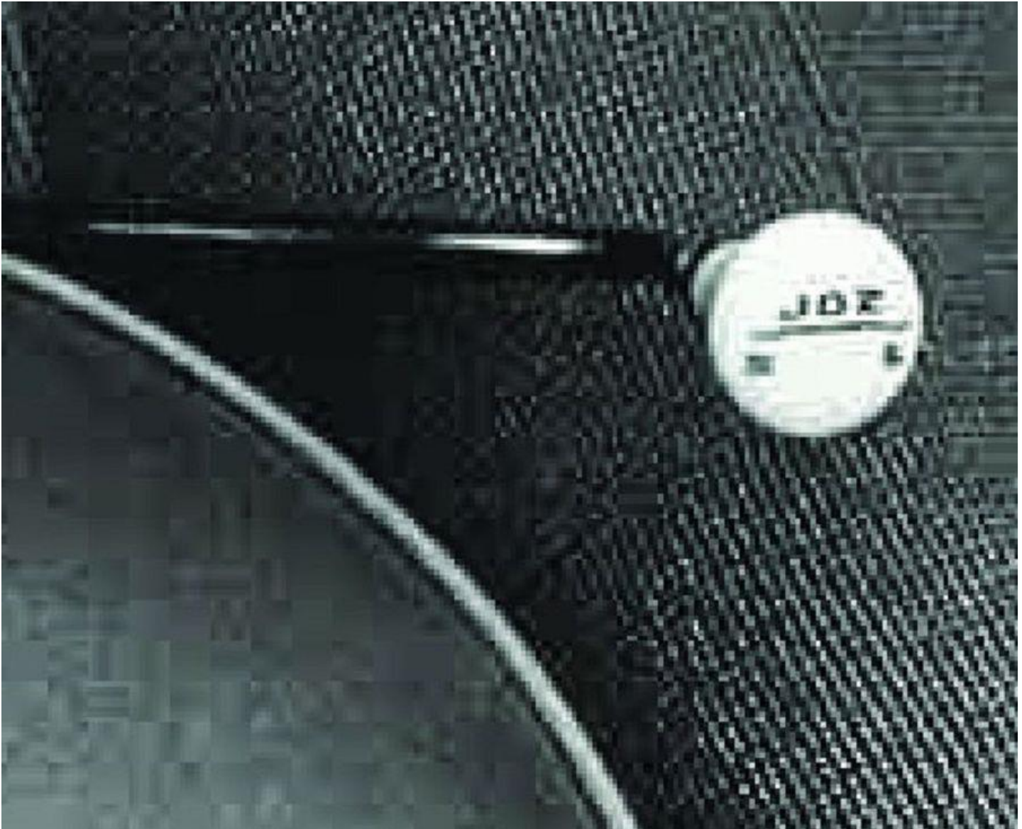
Baffling Powerglide control comes out of side of tunnel-like early Austin-Healy shifters.
