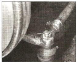
This is the tie rod end and is used for setting the toe on these early Corvettes. The tie rod end itself is a ball socket arrangement that should be checked for wear by having a friend turn the steering wheel while you watch for play in the joint. In order to adjust the toe on the car loosen the nut on the sleeve clamp and then turn the tie rod. Make sure you loosen the inner clamp as well when you do this. That one is a little harder to reach since it's actually under the middle of the car.
