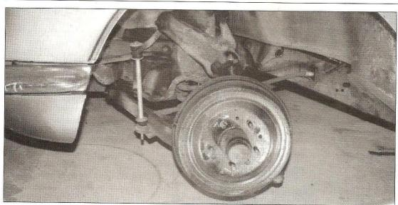
You're really looking at late-'40s technology here. This Corvette front suspension was taken right off a '53 Chevrolet sedan. These early Corvettes were designed before Chevrolet began using ball joints. The Corvette got ball joints 7 years after the sedans. We just kept going on with the old kingpin suspension.
