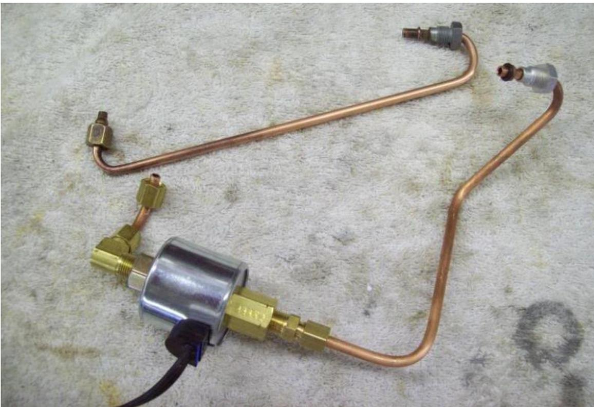
This picture compares the STOCK fuel line between the fuel meter and the fuel spider with John's solenoid and fittings that is available from John. The stock fuel line is completely replaced with the solenoid and fittings available from John DeGregory. I STRONGLY recommend installing one.
