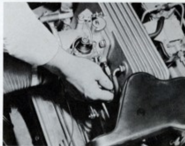
Fuel adjustment screw smooths out idle at proper speed.
