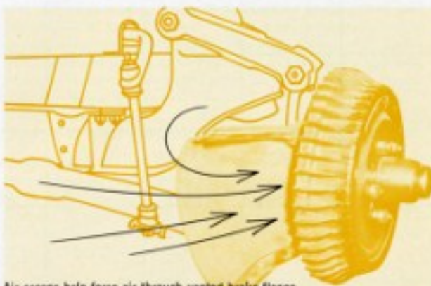
Air scoops help force air through vented brake flange.
