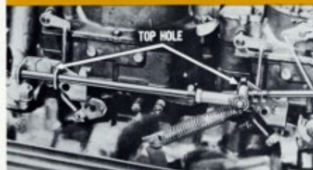
Corvette twin 4-barrel carburetion offers a choice of either simultaneous or progressive throttle opening. With linkage positioned as shown above, the front barrels of the rear carburetor open when front carburetor is at half throttle for smoother acceleration. In the lower illustration, the front barrels of both carburetors open simultaneously for maximum power. With either setting, rear barrels of each carburetor open only at higher engine speeds.
