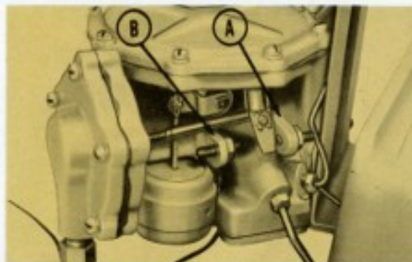
Mixture control stop screws are preset at factory and must not be adjusted without special equipment. Stop “A” is Rich, stop “B” is Lean.
